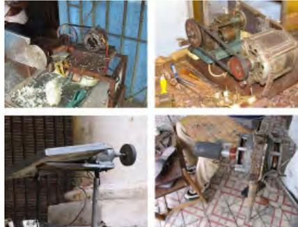
Images of "technological disobedience" collected by Ernesto Oroza: the electric engine from the widely-owned Soviet Aurika washing machine is commonly repurposed. Clockwise from left, in the photos above, the motors have been repurposed as coconut shredder, a key duplicator, a grinding wheel, and a shoe repair tool. Photos by Ernesto Oroza. Courtesy of the PBS NewsHour, 2015.
